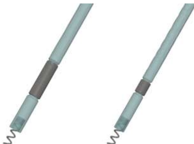
Figure 7: Lead designs tested for this report. Left: meshed from original Microport VEGA lead dimensions. Right: custom diameter and ring electrode size.
