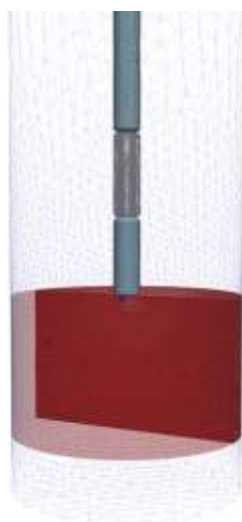
Figure 1: Example of computational mesh used to determine capture or non-capture. This specific mesh is built from the specifications of the Microport VEGA lead. Both translucent and solid red volumes depict the cardiac tissue, while the surrounding wireframe outlines the region simulating blood.
